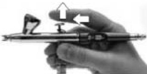
Move the trigger forward to stop paint
