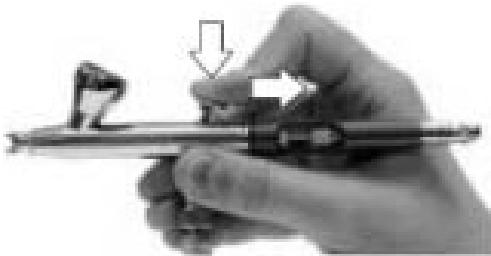
Press trigger to deliver air.
