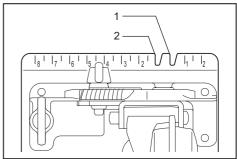
1. Cutting line (0° position) 2. Cutting line (45° position)
