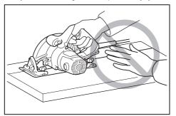
Never force the saw. Push the saw forward at a speed so that the blade cuts without slowing.
