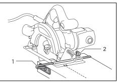
▶ 1. Rip fence (Guide rule) 2. Clamping screw
