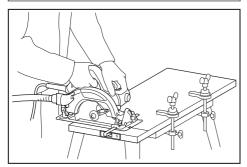
Hold the tool firmly. The tool is provided with both a front grip and rear handle. Use both to best grasp the tool.
