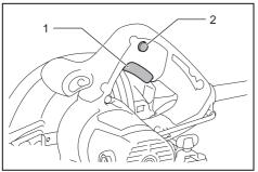
1. Switch trigger 2. Lock-off button
