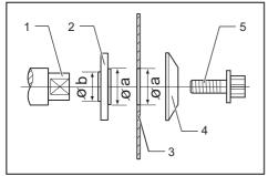
Mounting shaft 2. Inner flange 3. Circular saw blade 4. Outer flange 5. Hex bolt
