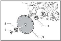
1. Hex bolt 2. Outer flange 3. Circular saw blade
