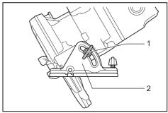
1. Clamping screw 2. Bevel scale plate
