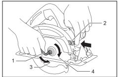
1. Hex wrench 2. Shaft lock 3. Loosen 4. Tighten
